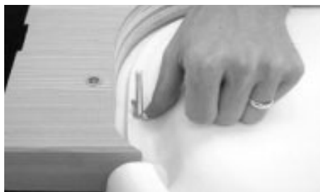
3 - The wing nut tightened on the threaded bar.
