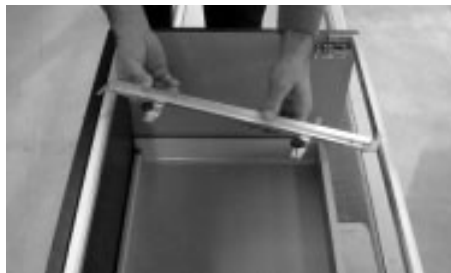
Position the support bar diagonally across the base unit.
