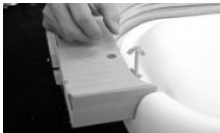
4 - Tighten the second wing nut, facing the opposite direction to the first, until it is parallel with the top.
