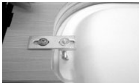
7 - Insert the washer into the threaded bar.
